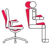
The dynamic motion enables a dynamic movement. In every position the posture is guaranteed a body opening angle of at least 90 degrees.
