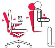
The individually adjustable counter-pressure of the backrest permits correct sitting for both light and heavy users.
