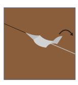
Go on removing the protective film over the lengths of sheets and smooth carefully the seams.
