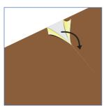
Remove the protective film from the adhesive tape (using a cutter blade for example).
