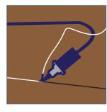
Groove first the seams. Then hot weld properly joins of Sarlon trafic modul'up.
