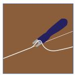
For a perfect finishing, trim off excess of welding rod in 2 steps.
