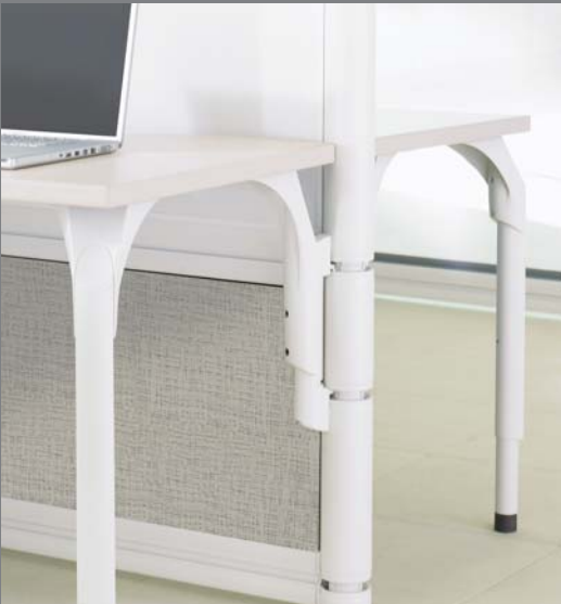
^ TABLE LEG AND BRACKET The Table Leg and Table Bracket provide an 8-inch height adjustable range for worksurfaces. The Table Bracket attaches to the post at any 15-degree angle to facilitate individual or shared support.
